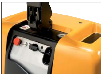
Pull-out charging cable. Start blocking during charging for high safety.
