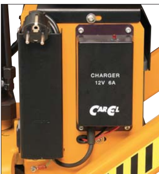
The electric scissor lift truck has a built-in charger as standard.
